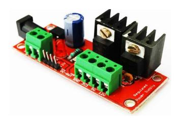
The regulated power supply accepts unregulated inputs from 9V to 15V AC or DC and gives regulated output of 3.3V, 5V and 12V suitable for projects which needs precise voltage to work. The input can come from step down transformer. Since board has Diode Bridge input polarity does not matter. All outputs are brought to screw terminal. There is also an unregulated output voltage to drive high current loads like relays and motors.
