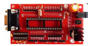
With this board you can develop and prototype with any of Microchip's 40 pin PIC microcontrollers. The RS232 driver on board allows easy connection with PC or other embedded hardware. The bridge rectifier allow this board to be powered with both AC and DC power supply adapters
