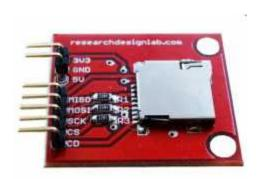
This is a wonderful little SD card interface module. It is easily interfaced as a peripheral to your module. Through programming, you can read and write to the SD card.All SD Card works on 3V interface so if your microcontroller is working on 3V you can use this board readily. The interface board provided is for microcontrollers running at 3V.
