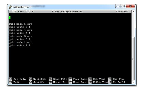
Here gpio mode X out will sets particular pin as output mode. And g3pio mode X 1 will writes 1 to the particular pin which will turns on the relay connected to the particular mode.
