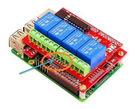
**Note 1:** Care should be taken while connecting AC voltages at the marked end. **Note 2:** Make sure that wires are not broken or wire skins are not out at the marked end.
