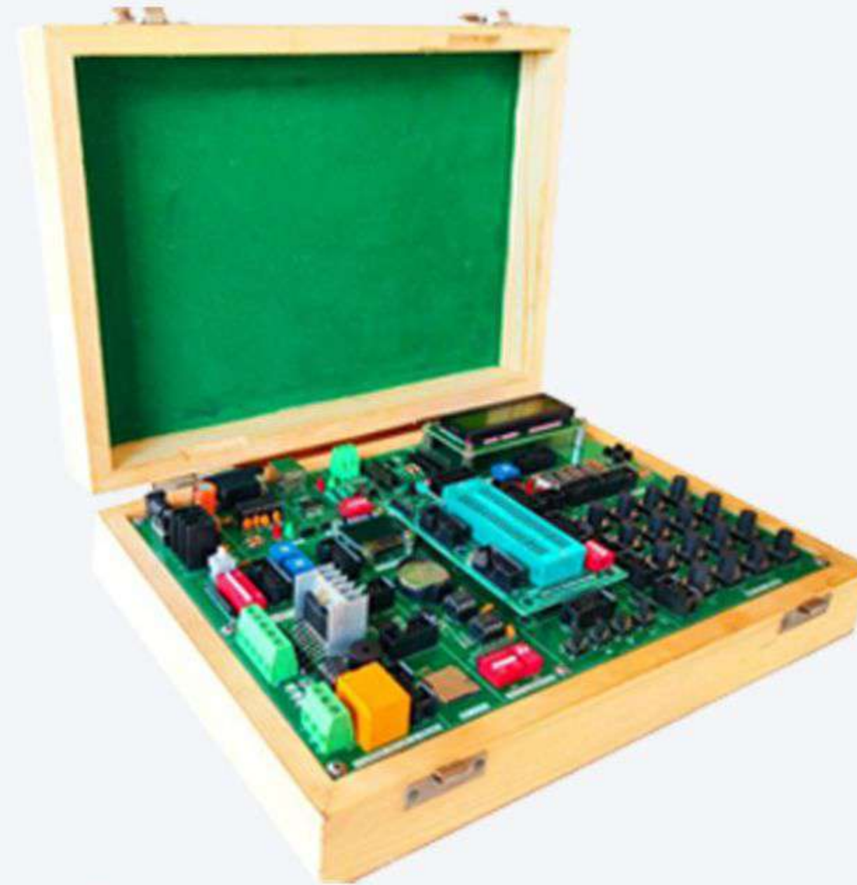
PIC Development Board- Trainer Kit Model No. : RDL740
