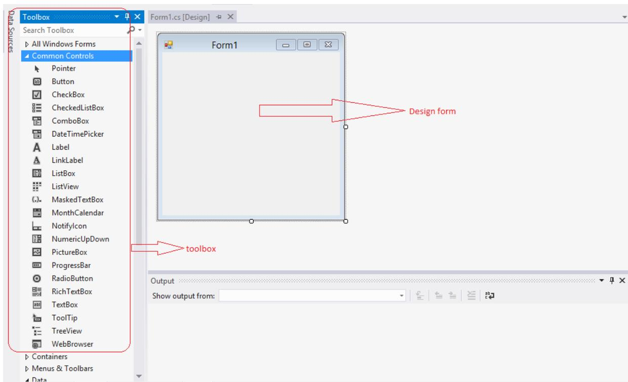
The following screenshot shows, making use of these toolbox controls for designing the user interface on DESIGN FORM.
