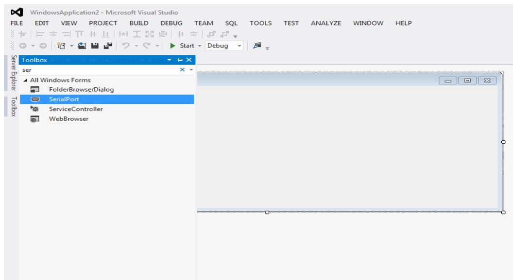
Shown in the above form before communicating with the particular hardware device we should add SerialPort tool from the Toolbox.
