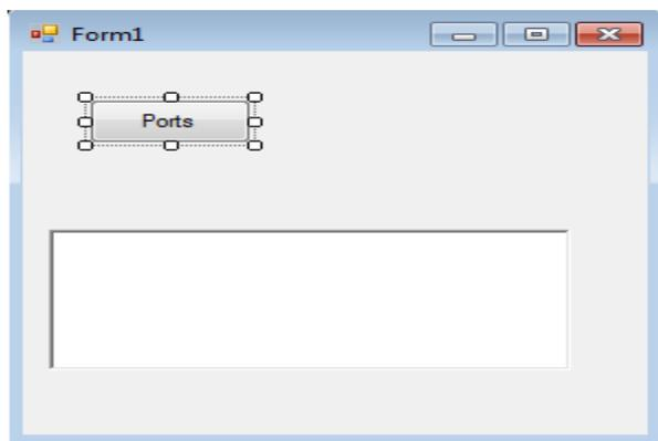
This is standard Windows Forms Application via File menu. To this add the button (name Ports) and a Rich Text Box. The button is called `btnGetSerialPorts` and the Rich Text called as `rtbIncomingData` (the name will become apparent later). The rich text box is used as it is more flexible than the ordinary text box. Its uses for sorting and aligning text are considerably more than the straight textbox.
