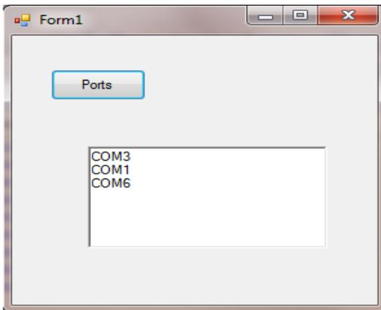
This shows all the devices that appear as com ports, a mistake to make is thinking that a device if plugged into the USB will appear as a COM Port.
