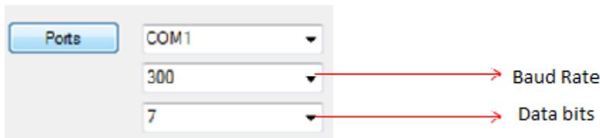
The next box is the number of Data bits, these represent the total number of transitions of the data transmission (or Tx line) 8 is the standard ( 8 is useful for reading certain embedded application as it gives two nibbles (4 bit sequences)).
