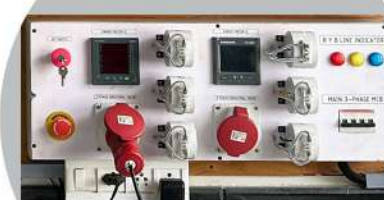
3 Phase Energy Meter with CT Coil
