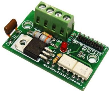
The board uses BTA12-600B, Triac suitable for general purpose mains power AC switching. They can be used as ON/OFF function in applications such as static relays, heating regulation or induction motor starting circuit. They are also recommended for phase control operations in light dimmers and appliance motors speed controllers.
