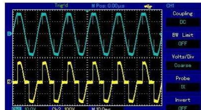
Fig B) shows 50% Dimming for given voltage when D3=0, D2=1, D1=1, D0=1
