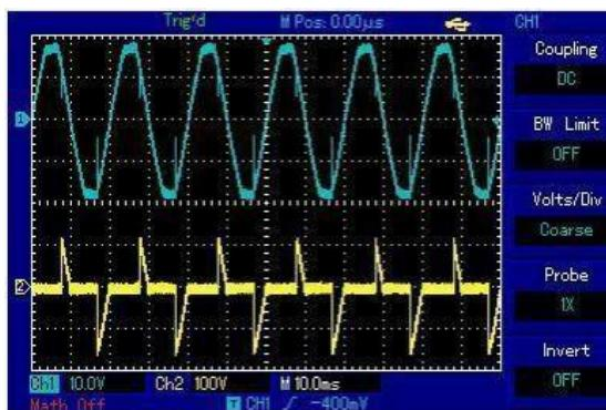
Fig A) shows 25% Dimming for given voltage when D3=1, D2=0, D1=1, D0=0
