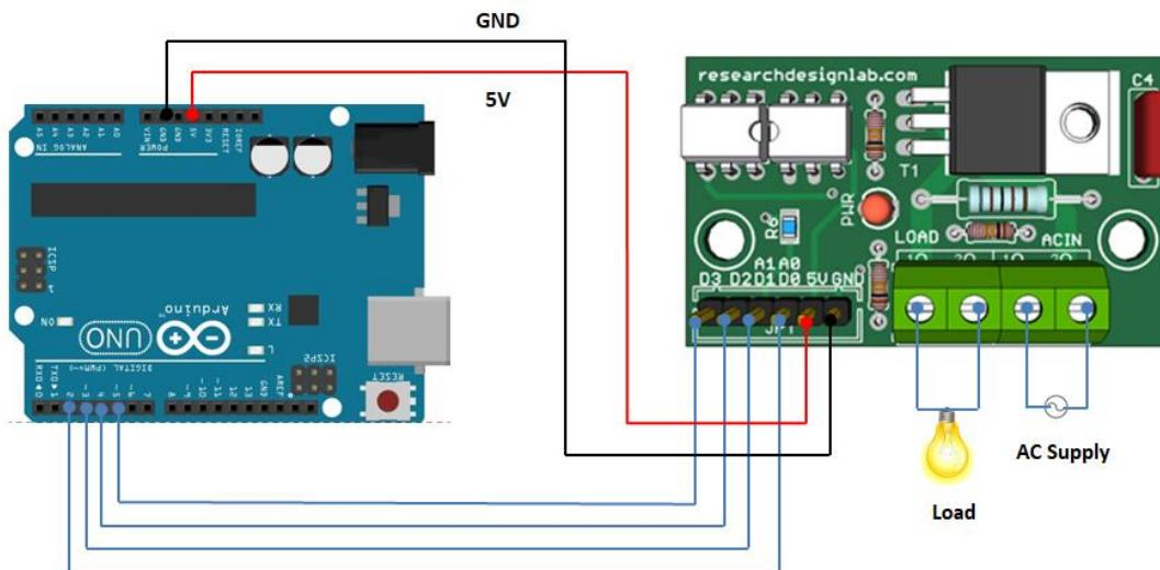
**Arduino program to control the dimmer 0-100% using simple IO handling**
