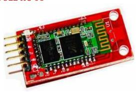
This module enables you to wireless transmit & receive serial data. It is a drop in replacement for wired serial connections allowing transparent two way data communication. You can simply use it for serial port replacement to establish connection between MCU or embedded project and PC for data transfer. This board operates on 5V and has LED indication and 3V regulator.
