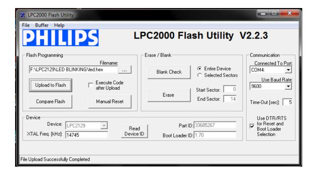
go to device manager and set the com port to com 4 or anything less than that because in Philips software we can select com from 1 to 5 only
