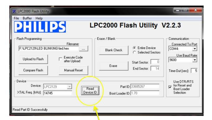
Click on Read device to check if the arm is connected properly or not
