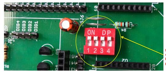
Make the dip switch on before burnig the program
